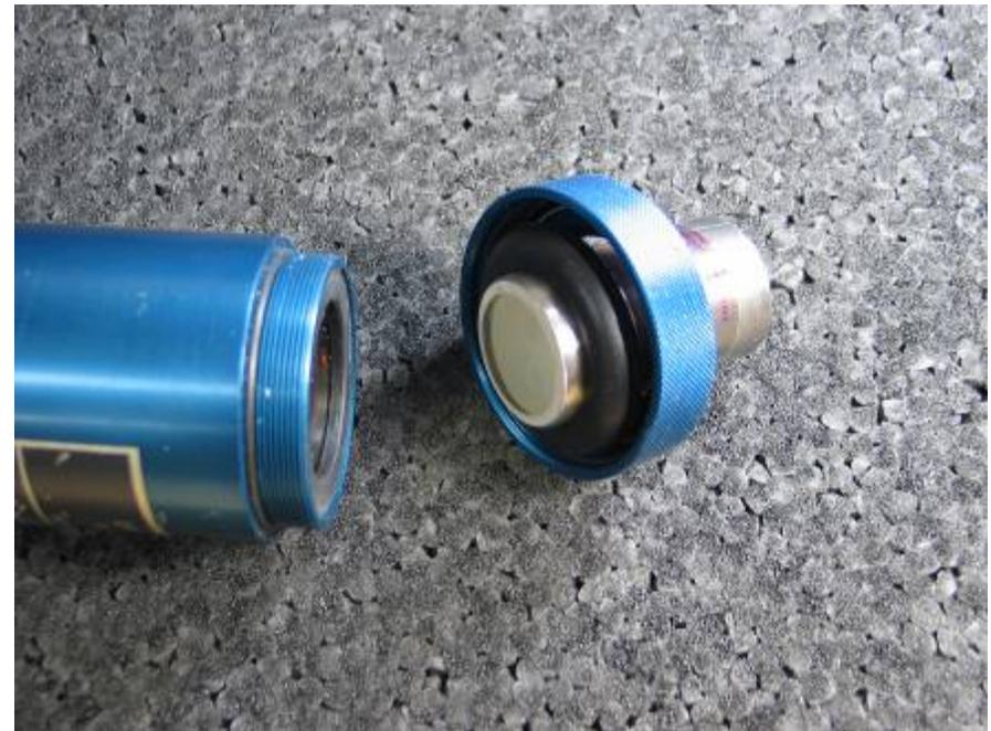
Coat the PMT face with index-matching gel and screw cap
