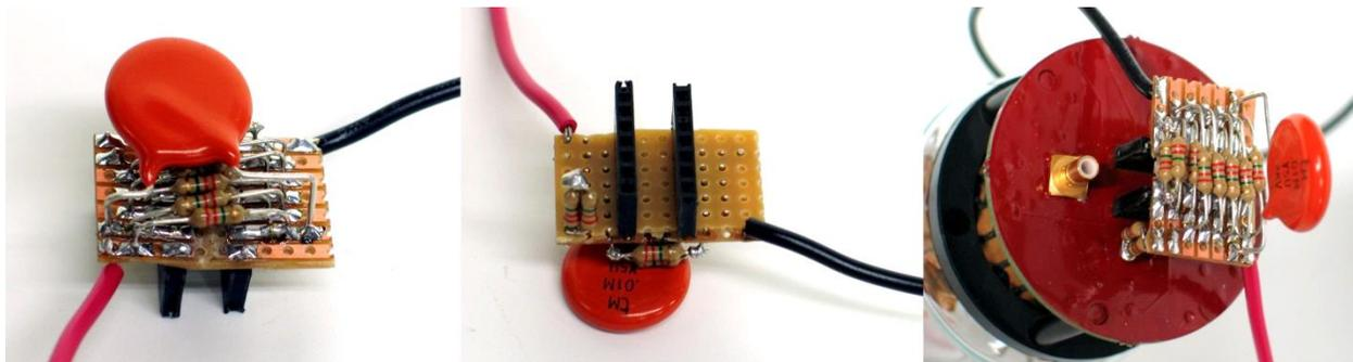
Figure 5 – Voltage divider network for the XP2422/SN PMT
