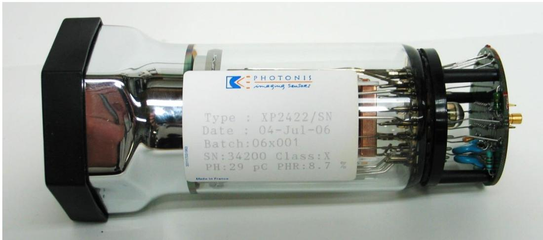
Figure 1 – New XP2422/SN photomultiplier tubes that were meant for medical gamma cameras are available at low cost from Sphere Research in Canada.
