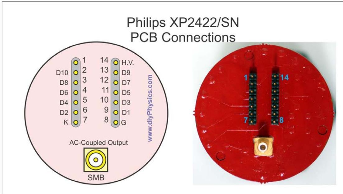
Figure 3 – Identification of connectors in the PCB of the Photonis XP2422/SN PMT assembly.
