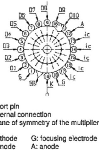
Figure 4 – Flying-lead pinout of the Photonis XP2422 PMT. The reference for numbering is one short pin that barely protrudes from the plastic retainer.
