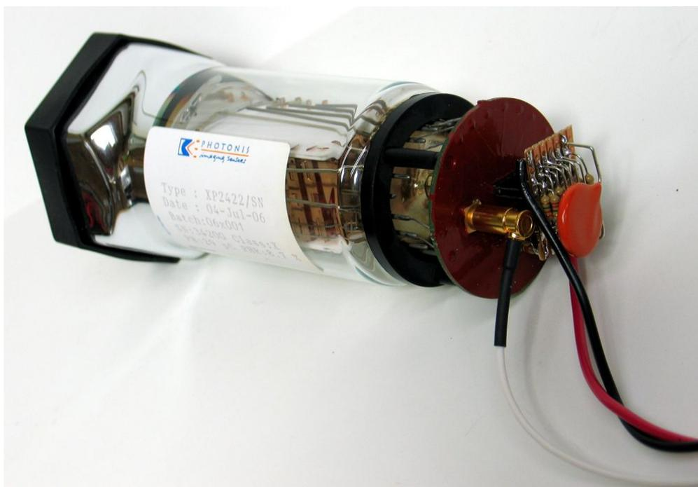
Figure 6 – Three cables connect the PMT assembly to an external +1,250V power supply and a scintillation processor: a HV reference wire, a high-voltage wire and a coax cable terminated by an SMB connector.
